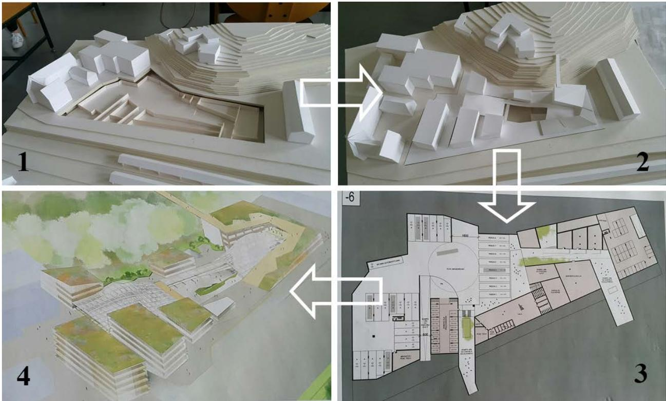
Figure 3: Results of the synchronous method of teaching architectural design: 1) matrix model of the site and its context. 2) mockup as the initial stage of the project development. 3) floor plans with details. 4) axonometric presentation with suggested façades and landscape solutions.
